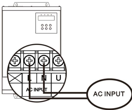
4. Make sure the wires are securely connected.
