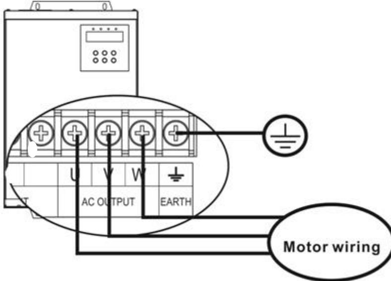
3. Make sure the wires are securely connected.
