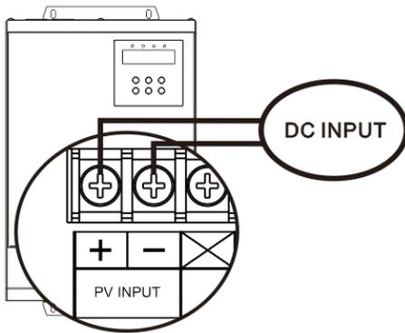
3. Make sure the wires are securely connected.
